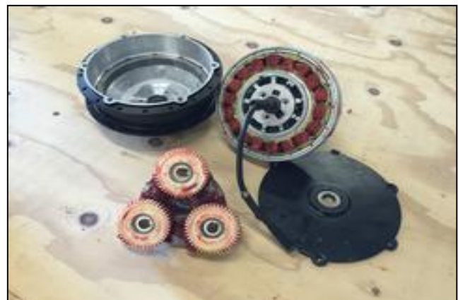
Fig 1: Geared Motor (500 W)
